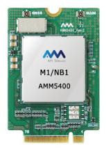
AM Telecom's AML540/AMM5400 supporting both Cat. NB1(NB-IoT) and Cat. M1 is the state-of-the-art telecommunication module for a narrow band IoT based service, and it adopted Qualcomm IoT-dedicated chipset which fully supports both Cat. NB1 and Cat. M1 in one single module based on 3GPP Rel 13. It helps your rapid and simple implementations on low power IoT services by incorporating with optimal networks for customers in various industry segments.
